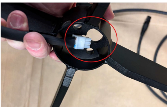
Image 5. The Molex connector of the extension cable is routed through the cross-type bottom plate of the leg
