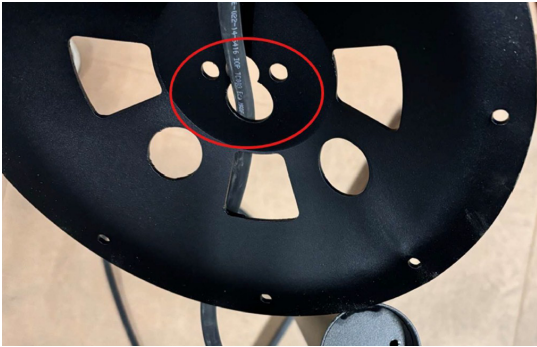
Image 7. The extension cable's Molex connector is routed through the leg top flange.
