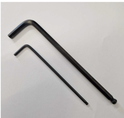
Image 4. A 3 mm and a 6 mm hex key are required for the final assembly.
