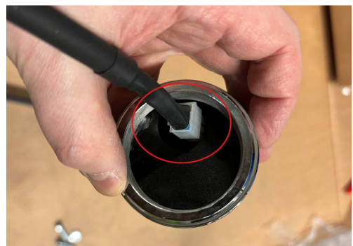
Image 6. The Molex connector of the extension cable is routed through the leg pipe
