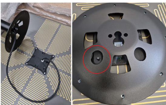
Image 12,13. The PCB power button and LED indicator are visible through the left circular opening
