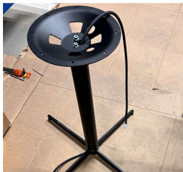
Image 10, 11. The fully assembled leg unit with integrated extension cable. The power cord is connected to the PCB.
