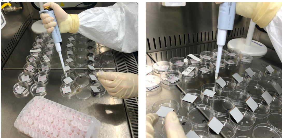
Figure 5: Analysed surfaces inoculated with droplets loaded with (SARS-CoV-2) virus.
